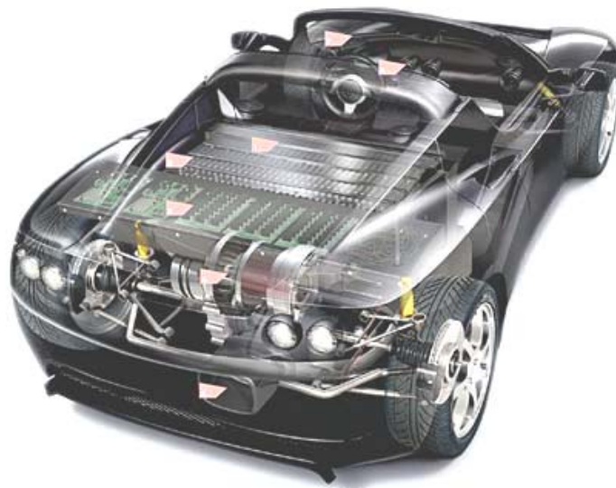
Figure 9: Tesla Roadster Cross Section (Courtesy: Treehugger)
