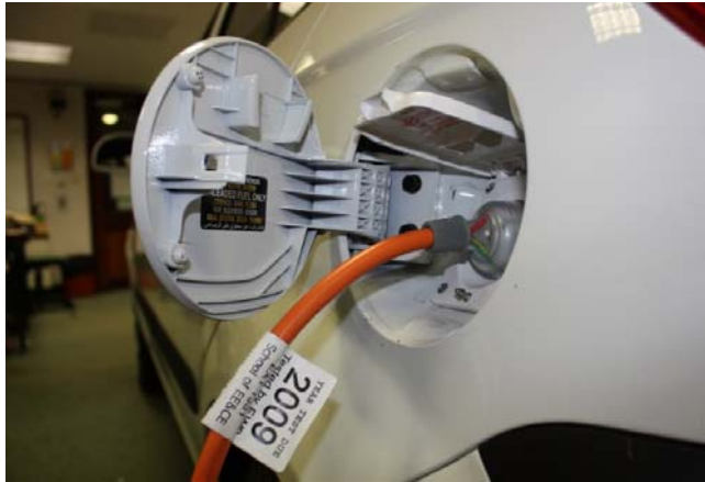
Figure 35: Charging cable connected to Recharging plug in fuel door.
