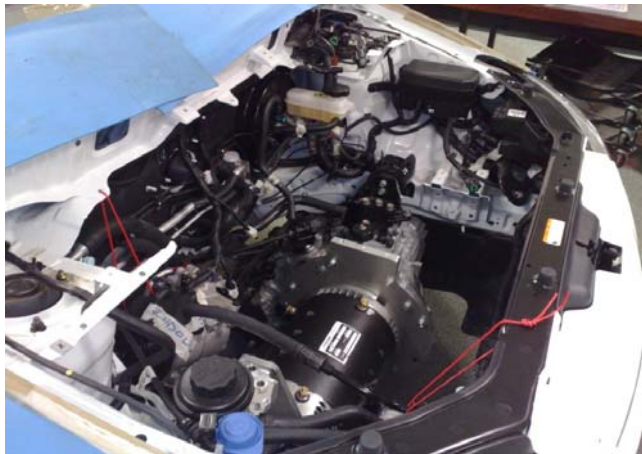
Figure 34: Cleared Engine Bay with DC Motor installed.
