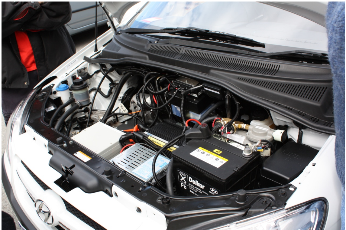
Figure 5.3 Electric systems installed in the Hyundai Getz
