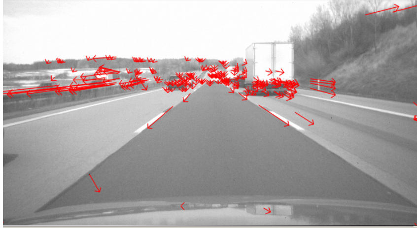
Figure 6.7: Flow vectors detected with Lucas and Kanade and pyramid images.
