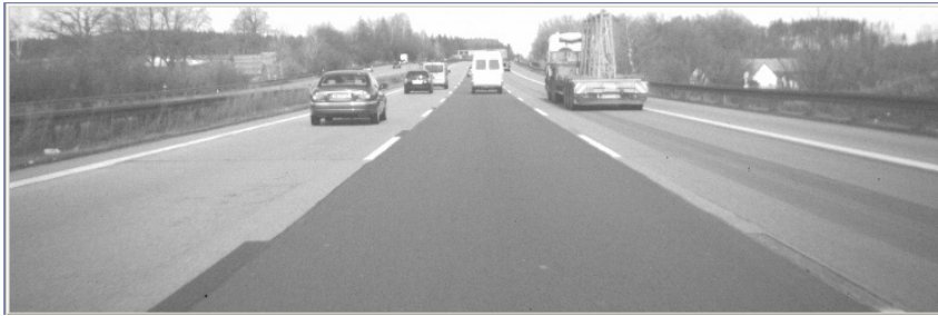
Figure 6.2: Image where upper part (the sky) and lower part (the car's front lid) have been clipped
