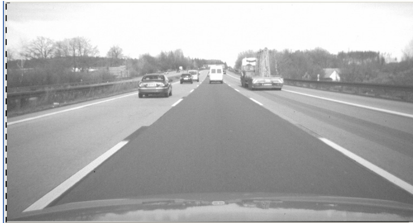
Figure 6.1: Unprocessed raw image data, taken by a camera mounted behind the car's windshield
