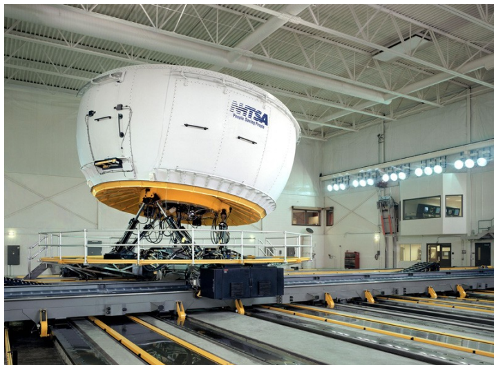
Figure 2.2: The NADS 1 simulator and its 13 degrees of freedom platform [13]
