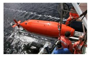
FIGURE 2.2: Deep water environment AUV, HUGIN 3000 Model [9].
