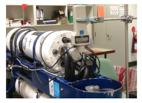
FIGURE E.3: An optical tachometer was used to measure the revolutions of the propellers
