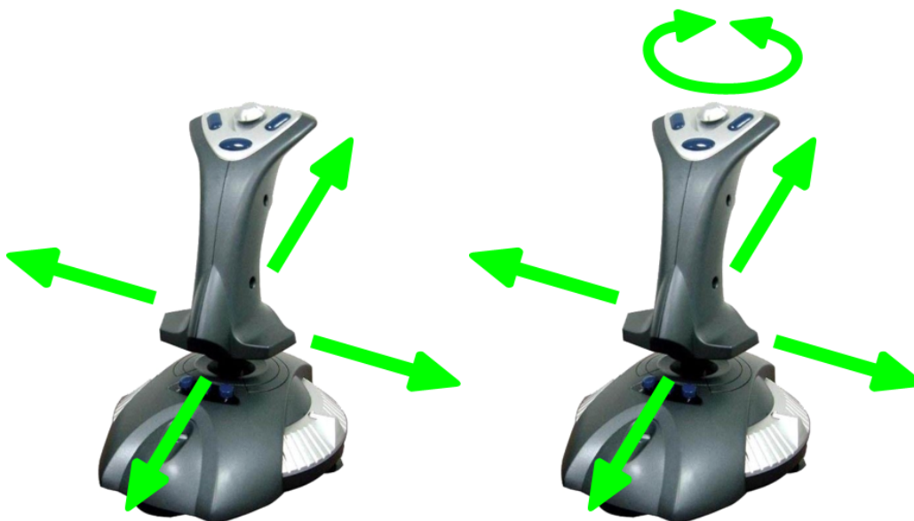
FIGURE 5.1: A 2 axis joystick compared to a 3 axis joystick
