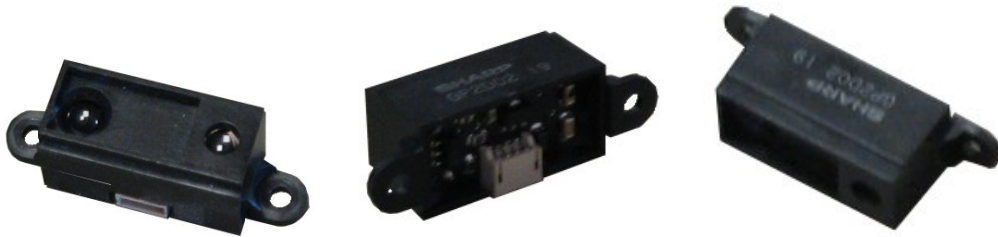
FIGURE 3.8: Position sensitive devices (PSDs)
