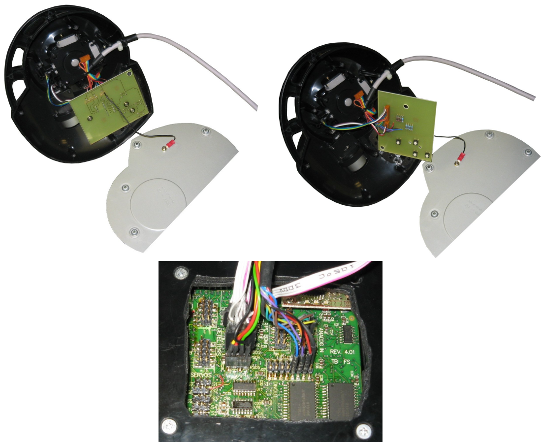
FIGURE 5.4: The new joystick circuit
