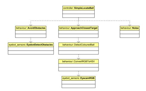
Figure 4.4: Relationships between schemas and controller in the LocateBall task
