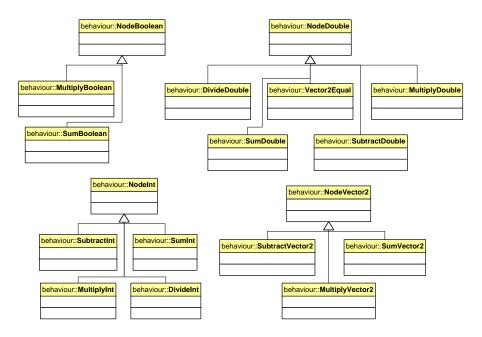
Figure A.2: Class hierarchy of the operator nodes provided by the framework
