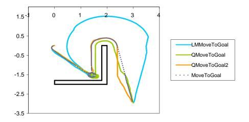
Figure 6.11: Path traces for each controller in dead-end scenario one
