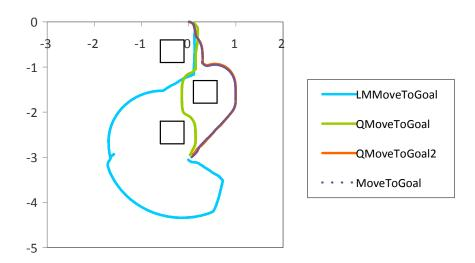
Figure 6.10: Path traces for each controller in cluttered environment two
