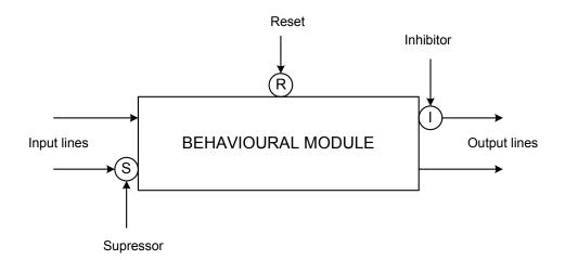
Figure 3.3: An augmented finite state machine purposed for subsumption
