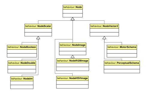
Figure A.1: Class hierarchy of the primitive types of the framework
