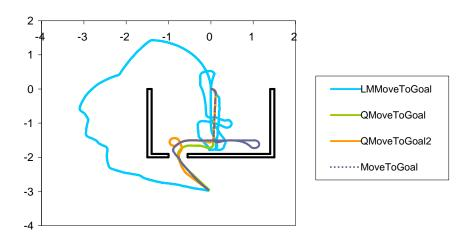
Figure 6.9: Path traces for each controller in cluttered environment one
