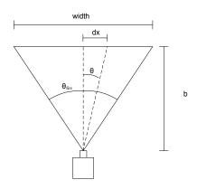
Figure C.2: Geometry used to calculate angle of an object
