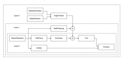
Figure B.5: Control system using self-preservation and task-oriented layers
