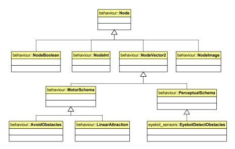
Figure 4.3: Simplified class diagram showing relationships between selected schemas
