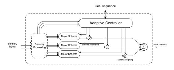
Figure 1.1: Adaptive controller concept schematic
