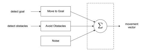
Figure 5.3: Behavioural assemblage used in the QMoveToGoal controller
