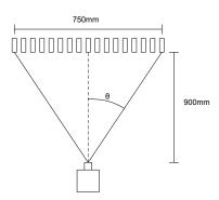
Figure C.1: Experiment configuration for determining field of view of the camera
