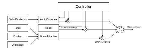
Figure 5.2: Navigation task schemas coupled with an adaptive controller
