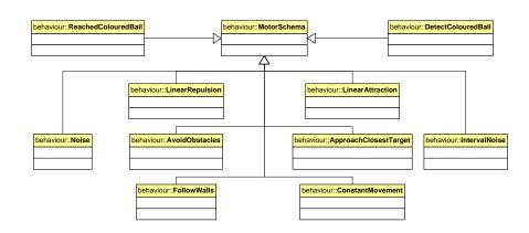
Figure A.3: Hierarchy of the general purpose motor schemas created for the framework
