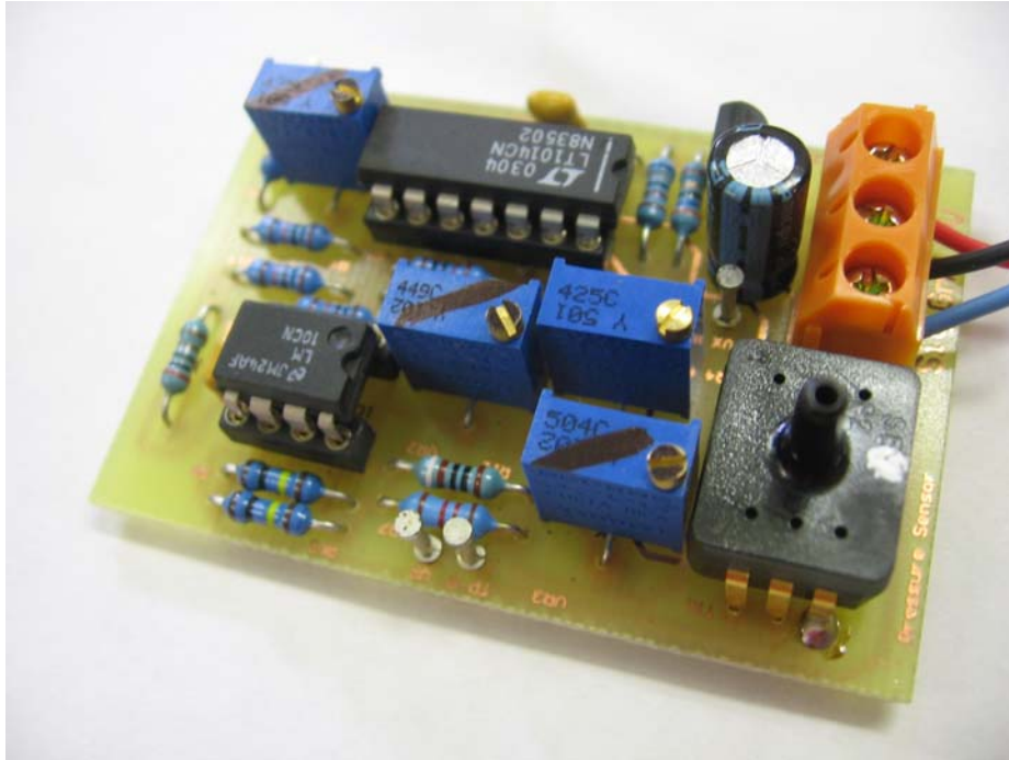
Figure AI-1: Circuit board with pressure sensor
