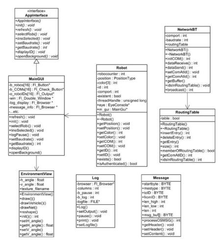
Figure 4.15: Class diagram
