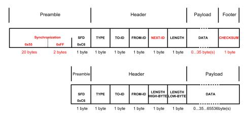
Figure 3.3: Old vs. new frame structure
