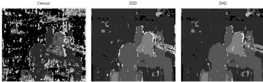
Figure 18: Comparison of the depth maps of Census (left), SSD (center) and SAD (right)
