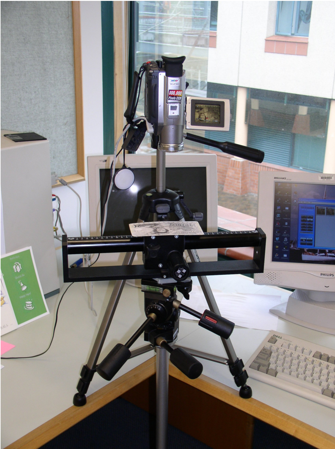
FIGURE 4.4: Camera and rack and pinion tripods setup
