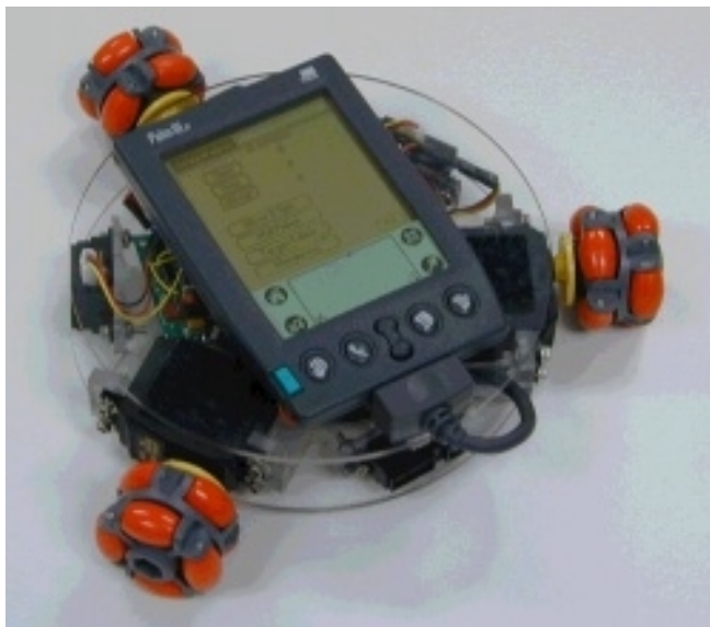
Figure 2.1.4 The Palm Robot Kit, using Three mecanum wheels.
