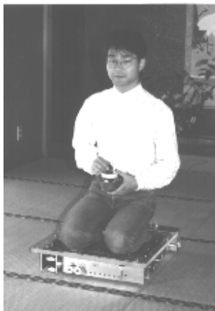
Figure 2.1.2 The Vuton uses a revolutionary form of caterpillar track, enabling a very large payload capacity.
