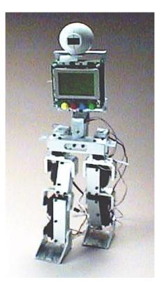
Figure 3.5: A photograph of the constructed robot. Overall the robot characteristics were as planned except for the COM. However the balance was found to be exceptional, with the robot being able to statically balance quite stably without actuation in an upright position.
