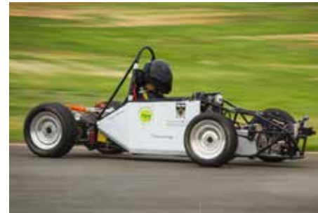
Autonomous SAE Electric car Twin DC drive motors, 13kW, 48V, 4.3kWh, drive-by-wire, laser scanner, GPS, IMU, camera.
