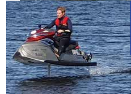
REV Waveflyer Twin 5kW shrouded DC motors, 48V, 2kWh, 30min. drive-time.
