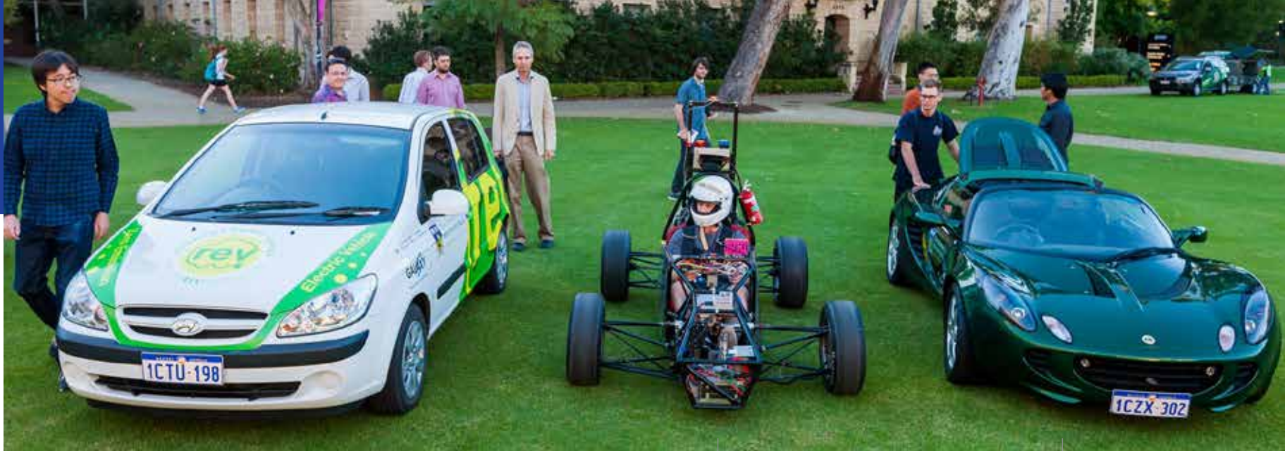
REV Eco Electric conversion of Hyundai Getz: DC drive system, 28kW, 144V, 13kWh, 80km range.
