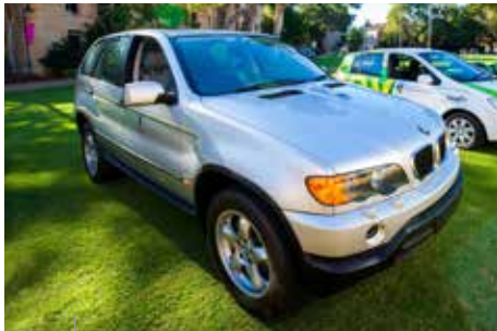
Autonomous BMW X5 Drive-by-wire, laser scanner, GPS, IMU, camera.
