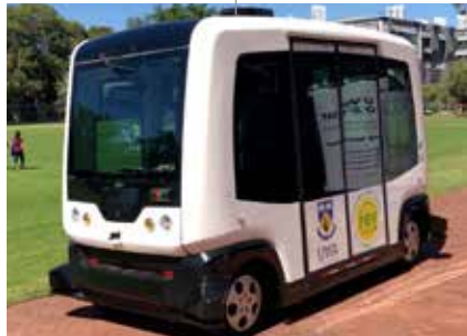
Autonomous Electric Shuttle Buses—nUWay 48V, 15.36kWh, 8 Lidars, 2 cameras, IMU, RTK-GNSS.
