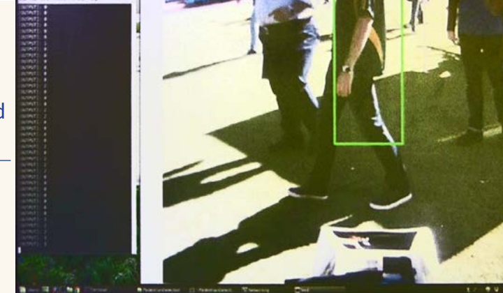
Above: Pedestrian detection using OpenCV. Based on the pedestrian's position in the frame, the vehicle is able to react and steer away from the pedestrian.
