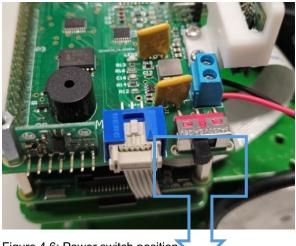
Figure 4.6: Power switch position
