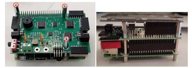
Figure 4.5 Raspberry pi attached to IO board with 15mm hex standoffs on top and with display attached
