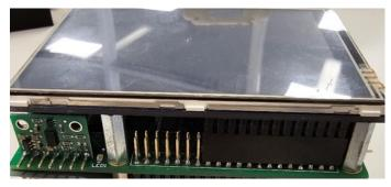
Figure 4.12. LCD Screen Connected to IO-Board
