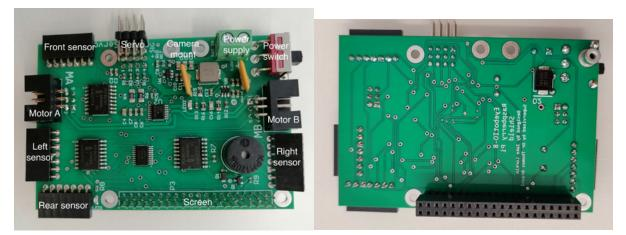
Figure 4.1: Connections on EyeBot-8 board top and bottom
