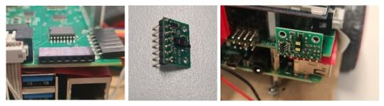
Figure 4.11: PSD Sensor socket (left). PSD Sensor (middle). connected PSD Sensor (right)
