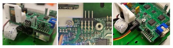
Figure 4.10: Camera mount (white 3D) and servo connector front (top left) and above (top right). connected Servo (bottom) with Brown = Ground, Red = Power and Yellow = Signal
