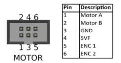
Figure 4.8: EyeBot8 motor and encoder connectors
