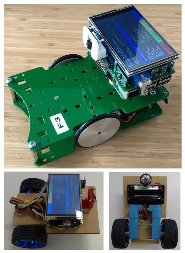
Figure 6.1: SoccerBot and EyeCart mobile robots with EyeBot-8 board
