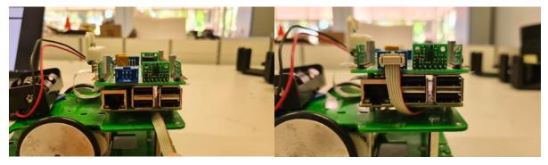
Figure 4.9: Motor port without (left) and with (right) motor connected.
