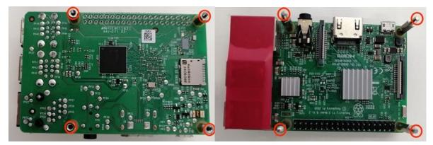
Figure 4.4 Raspberry pi with 8mm hex standoff on back and with hex-stand-off on top
