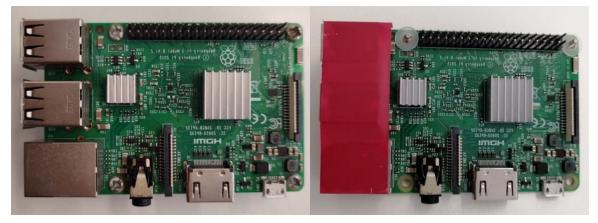
Figure 4.3 Raspberry Pi without and with insulation tape
