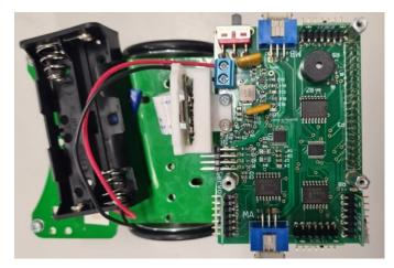
Figure 4.13: EyeBot-8 board mounted on robot without LCD screen
