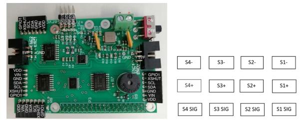
Figure 4.2: Full pin-outs and servo connector pins
