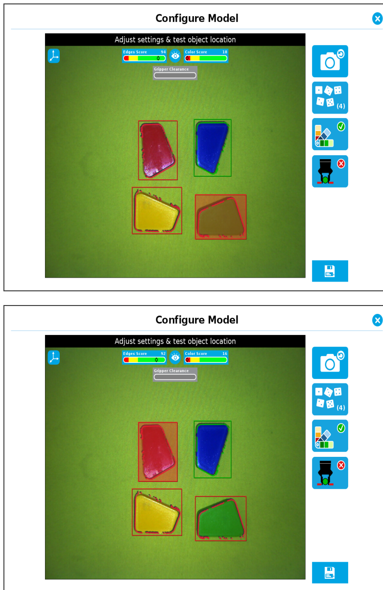
Fig. 4-51: Multiple objects found each with their selection rectangles and detection scores.
