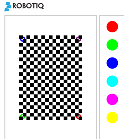
Fig. 4-8: Calibration board for UR3 Universal Robots models.
