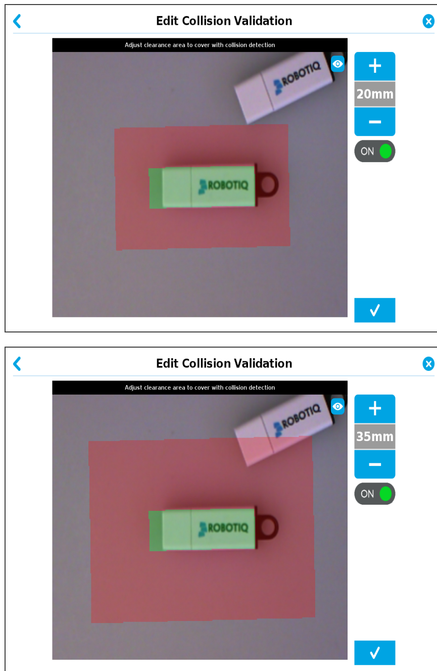
Fig. 4-57: Setting up the clearance perimeter.
