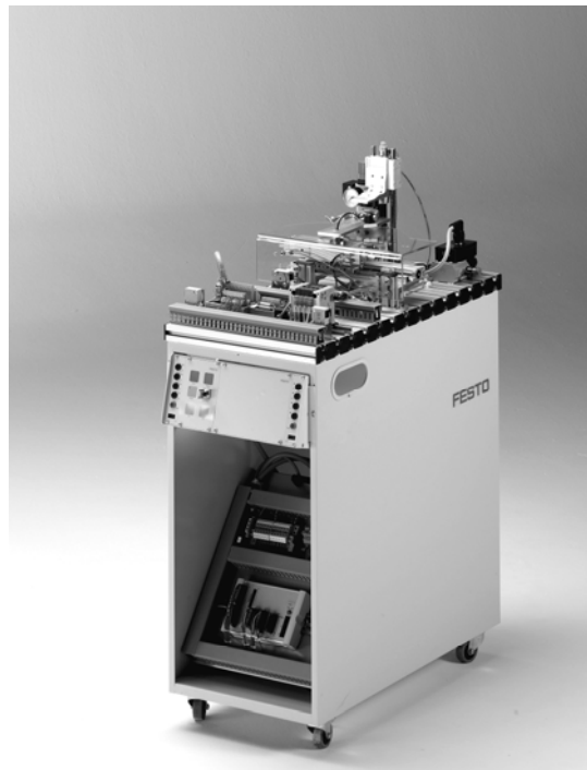
Fluidic Muscle Press station with trolley, control console and PLC board
