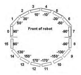
Fig. 2.1 The angular positions of the sonar sensors
