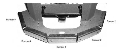
Fig. 2.3 Rear bumpers on the Pioneer robots
