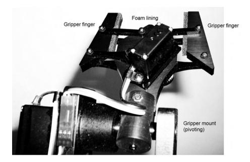
Fig. 2.4 5D arm gripper detail
