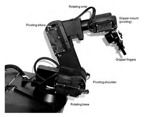
Fig. 2.5 The joints on the Pioneer
