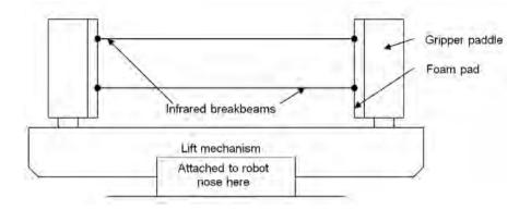
Fig. 2.6 The Pioneer 2D gripper
