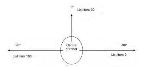
Fig. 2.2 Laser readings and their positions on the robot (181 readings)
